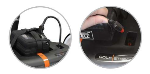
Place CaddyCell Lithium battery sideways in tray on the chassis. Secure with strap. Plug power connector into port on chassis. Once battery is plugged in, the Vision Screen will begin to flash and display "Power Off". This signals Golfstream is idle and not "Power On" yet.
